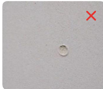
Surface too wet (2:55) ▶
